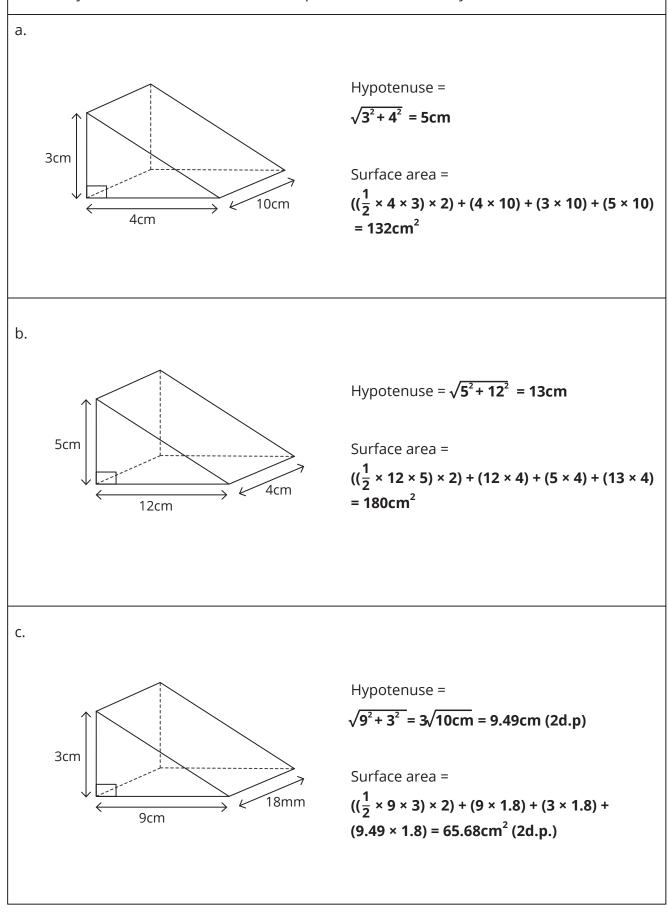
The diagrams show some prisms of which the cross-section is a composite shape.
